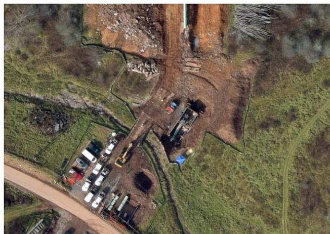
ACP STREAM CROSSING IN POCAHONTAS COUNTY. THE CROSSING DOES NOT CONFORM TO THE METHOD SPECIFIED IN APPROVED PLANS.
